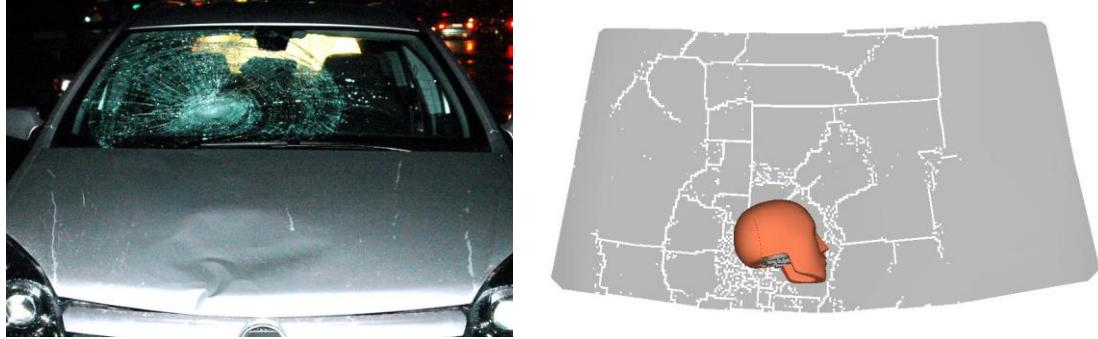
**Figure 14 Fracture pattern of windshield during accident photo (left) and a simulation (right)**
