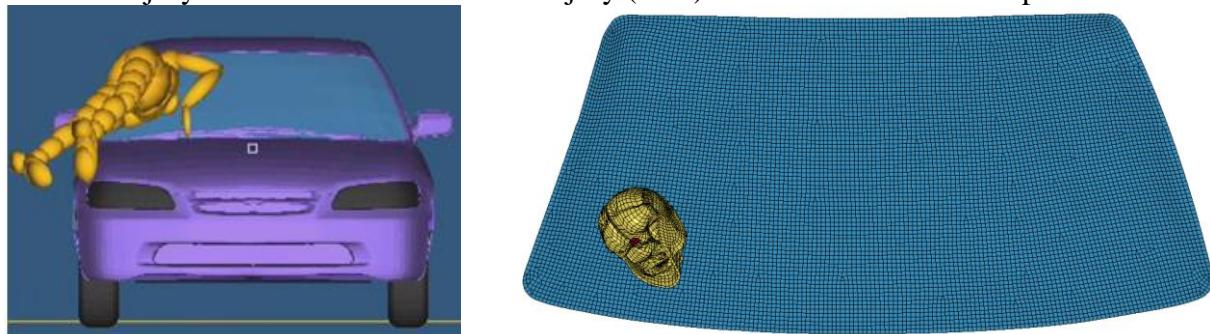
Figure.11 View of impact configuration involving windscreen in MADYMO and impact configuration in LS-DYNA.
